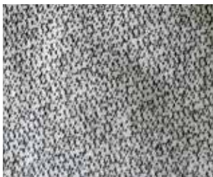
Fig. 3 Moiré free print with a RandomScreen® Eco - 125 mesh
